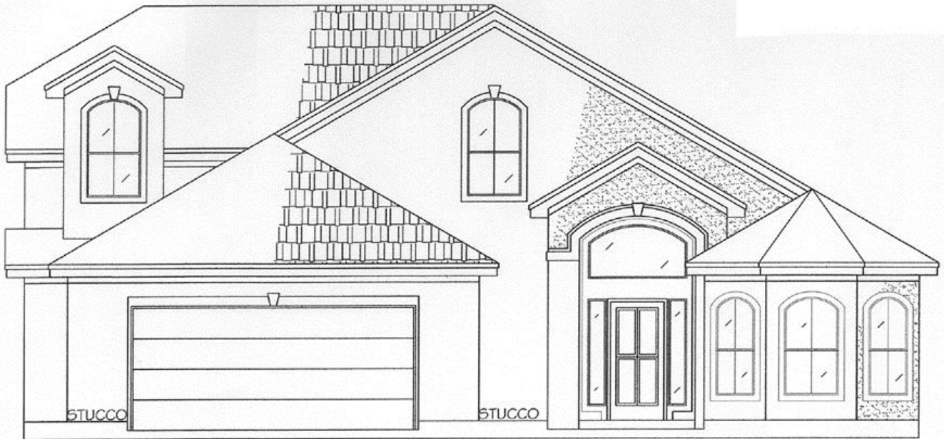
FRONT ELEVATION PLAN No. 2748-0203 4-BEDROOM | 1 1/2-STORY 2848 SQ. FT. LIVING AREA MONTE SMITH DESIGNS COPYRIGHT 2007
